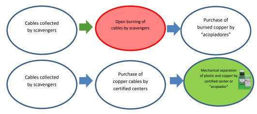
Figure 22: Current situation (above) and proposed system of collection and separation of cables (below).
