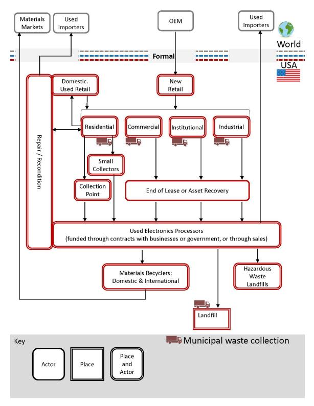
Figure 3: Diagram showing basic material flow stages for used electronics
